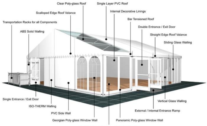
Steel Sub-frame Flooring with Timber Boards or Aluminium Cassette Flooring with Ply Boards
